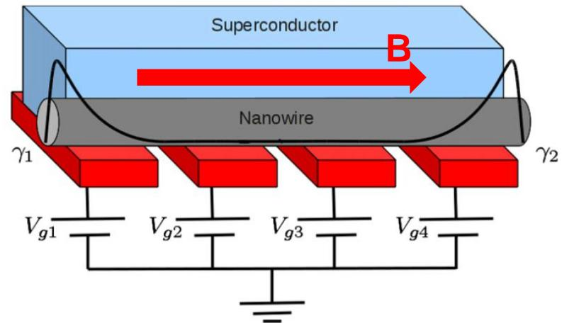
$$H_0(\mathbf{r}) = \frac{\mathbf{p}^2}{2m} - \mu + V(\mathbf{r}) + \alpha (\mathbf{E}(\mathbf{r}) \times \mathbf{p}) \cdot \bar{\sigma} + \frac{1}{2} g \mu_B \mathbf{B}(\mathbf{r}) \cdot \bar{\sigma}, \quad \xrightarrow{\text{transform}} H_0(x) = \frac{k_x^2}{2m} - \mu + \tilde{\alpha} k_x \sigma_y + \frac{1}{2} \tilde{B} \sigma_z$$
