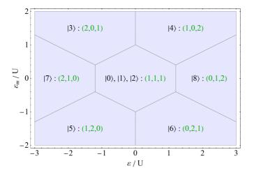
FIG. 1. Charge stability diagram: Lowest-energy charge states as functions of the detunings  $\varepsilon$  and  $\varepsilon_{\rm m}$  with  $U_{\rm c} = 0.2 U$ . In the absence of tunneling and hyperfine field, states  $|0\rangle$ ,  $|1\rangle$ , and  $|2\rangle$  are degenerate.
