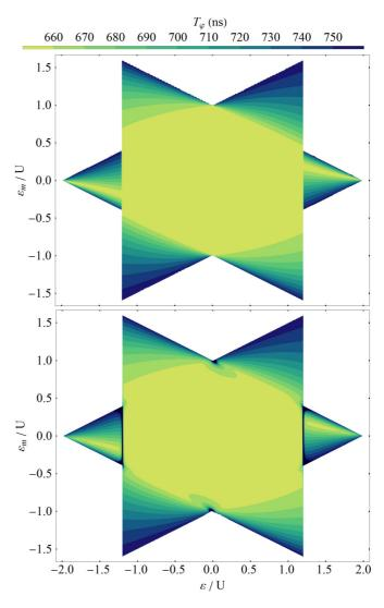
FIG. 4. Dephasing time in nanoseconds for realistic input parameters:  $U_c/U = 0.2$ ,  $t_1/U = 0.015$ ,  $t_r/U = 0.01$  and g = 2.0,  $\sigma_z = 15 \,\mu$ T, which corresponds to natural Si [23]. In the upper figure, the analytic formulas for  $T_{\varphi 0n}$  are evaluated, while in the lower figure, the numerical solution of the full problem is plotted, which is also accurate close to the borders, see the main text.
