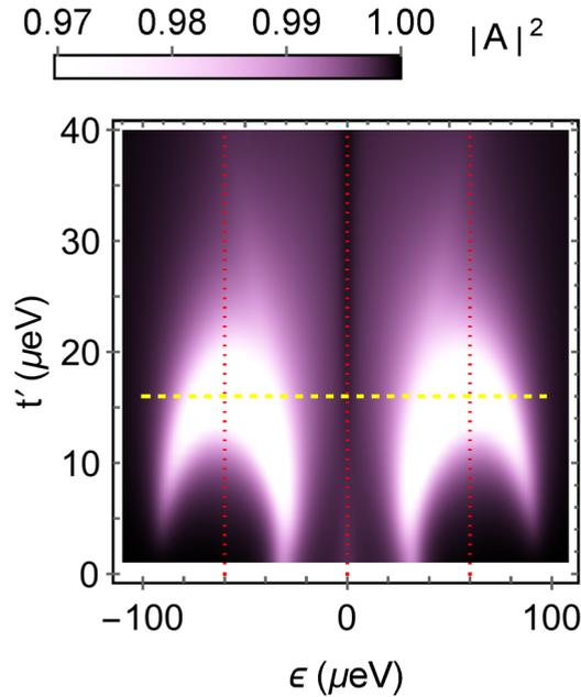
FIG. 5. Cavity transmission as a function of  $\epsilon$  and the intervalley matrix element  $t'$  for  $t \sim 0$ . Here we use  $E_L = E_R = 60 \mu\text{eV}$ , and  $f_0 = \omega_0/2\pi = 7.8 \text{ GHz} = 32 \mu\text{eV}$ ,  $\omega_R = \omega_0$ ,  $T = 250 \text{ mK}$ . The yellow horizontal line indicates  $t' = f_0/2$  where the double lines merge into single lines. The vertical red dotted lines indicate the anticrossings in the DQD spectrum (cf. Fig. 1).
