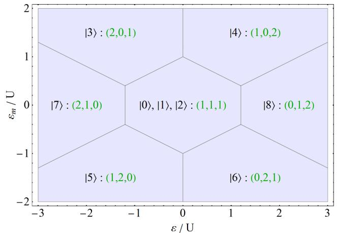
FIG. 1. Charge stability diagram: lowest-energy charge states as functions of the detunings  $\varepsilon$  and  $\varepsilon_m$  with  $U_c = 0.2U$ . In the absence of tunneling and hyperfine field, the states  $|0\rangle$ ,  $|1\rangle$  and  $|2\rangle$  are degenerate.
