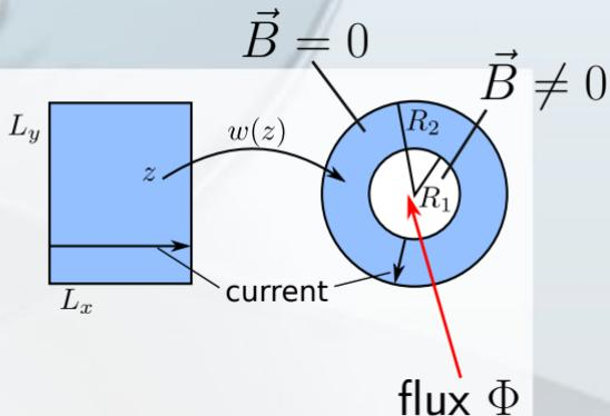
$$T = 4 \cdot \left| \frac{\psi_1^C(x=0, y)}{\psi_1^C(x=L_x, y)} + \frac{\psi_2^C(x=0, y)}{\psi_2^C(x=L_x, y)} \right|^{-2} e^{-q(\phi(R_1) - \phi(R_2))} e^{k_y L_x}$$
